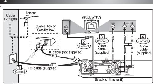
Both A/V and RF cables must be connected to the TV for operation. See front page of the Owner's Manual for the connection with the RF modulator.
